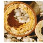
Calcifications: The minerals present in the water, especially limestone and magnesium, accumulates continuously in the walls of the circuits. The result is continuous loss of flow till complete obstruction.
